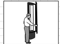
Open display panel door and locate translite held inside display face.
