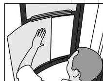
Gently insert translite into top and bottom retention channels on the side closest to you.
