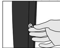
Insert display panel key (provided with unit) into locks and turn clockwise to unlock.
