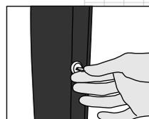
Insert display panel key (provided with unit) into locks and turn clockwise to unlock.
