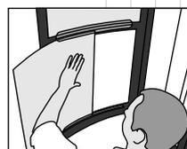
Gently insert translite into top and bottom retention channels on the side closest to you.
